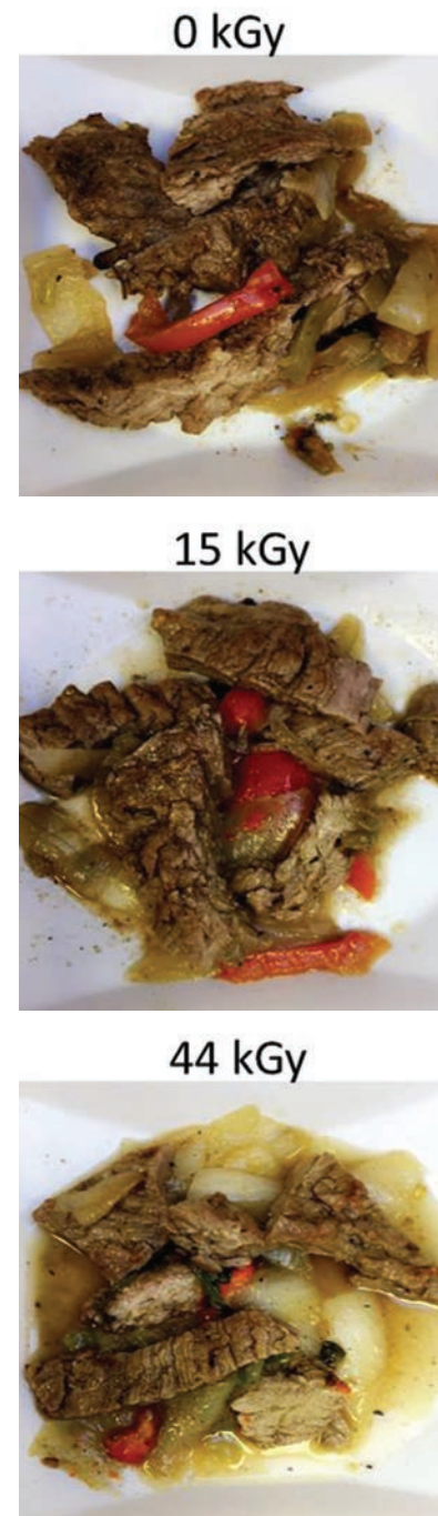
Figure 2. Beef fajitas processed with increasing eBeam doses. With each increased dose, color appears to fade and moisture is released from the food.
